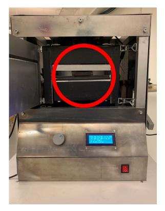
Figure 7: HTC-testing setup, the red circle highlights the material specimen and its placement for the test.
