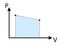
Figure 14: A schematic figure over a P-V diagram where the work is the area under the function. The figure is only for an expansion of the WGV and the same principal applies for the compression.
