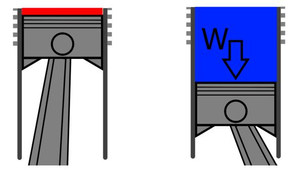
Figure 6: Simplified 2-stroke cycle. Compressed fluid in a closed volume with high pressure and temperature on the left. When the fluid expands it presses on the piston with a force and generates mechanical work.
