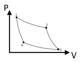
Figure 4: P-V diagram of an ideal Carnot cycle.
