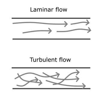
Figure 5: Illustration of laminar and turbulent flow in a tube.
