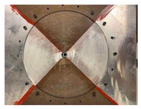
Figure 9: Image of the conducting and heating fins of the GREC. The brown fins are the insulating fins made of FRP and the aluminium fins are the conducting fins.
