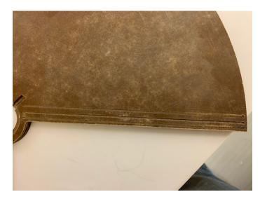
Figure 13: Slits on the rotating shutter. Three slits are placed on each side of the WGV and on both sides of the RS.
