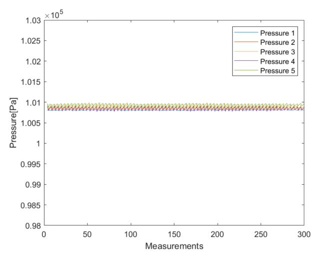
Figure 15: A graph over the pressure from the different pressure sensors which is presented under method. The x-axis is the measurements, i.e the testing was done with 300 measurements per sensor. The y-axis is the measured pressure from the sensors.
