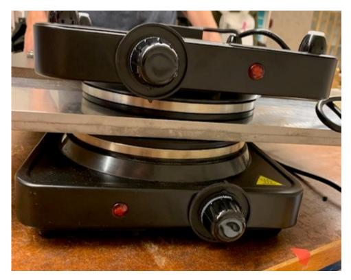
Figure 10: The heating source method setup consisting of two hot plates, one on each side of the heating fin.
