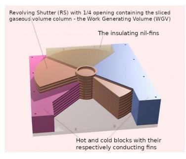
Figure 2: Cutout of the GREC, shows how several layers of RS can be used to increase the volume of the GREC engine.
